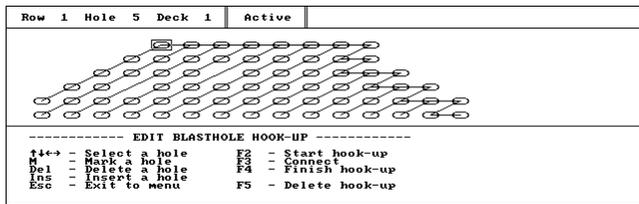
Design any pattern with Electric or Non-Electric Initiation up to 40 holes per row, 15 rows and 10 decks per hole.
