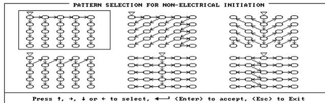
A unique feature allows the user to define how many charges may overlap without causing problems. The program will determine overlaps if they exceed the criteria entered by the user. The probability of overlap, when calculations include cap scatter (tolerance) is also reported.
